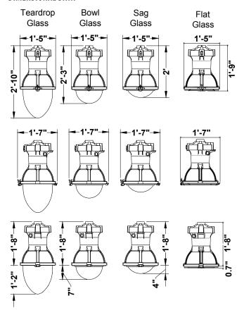
**Optional NEMA** Turn-Lock **Photocontrol** 1.50" NPT Receptacle Tool-less Pendant Mount (P) latch **Quick Lock** Stem Mount (S) Wiring Hinge Chamber Uplight Refractor (Optional) Stainless Steel Latch Hinge Sag Electrical/ Glass Reflector **Teardrop Glass** Assembly -
