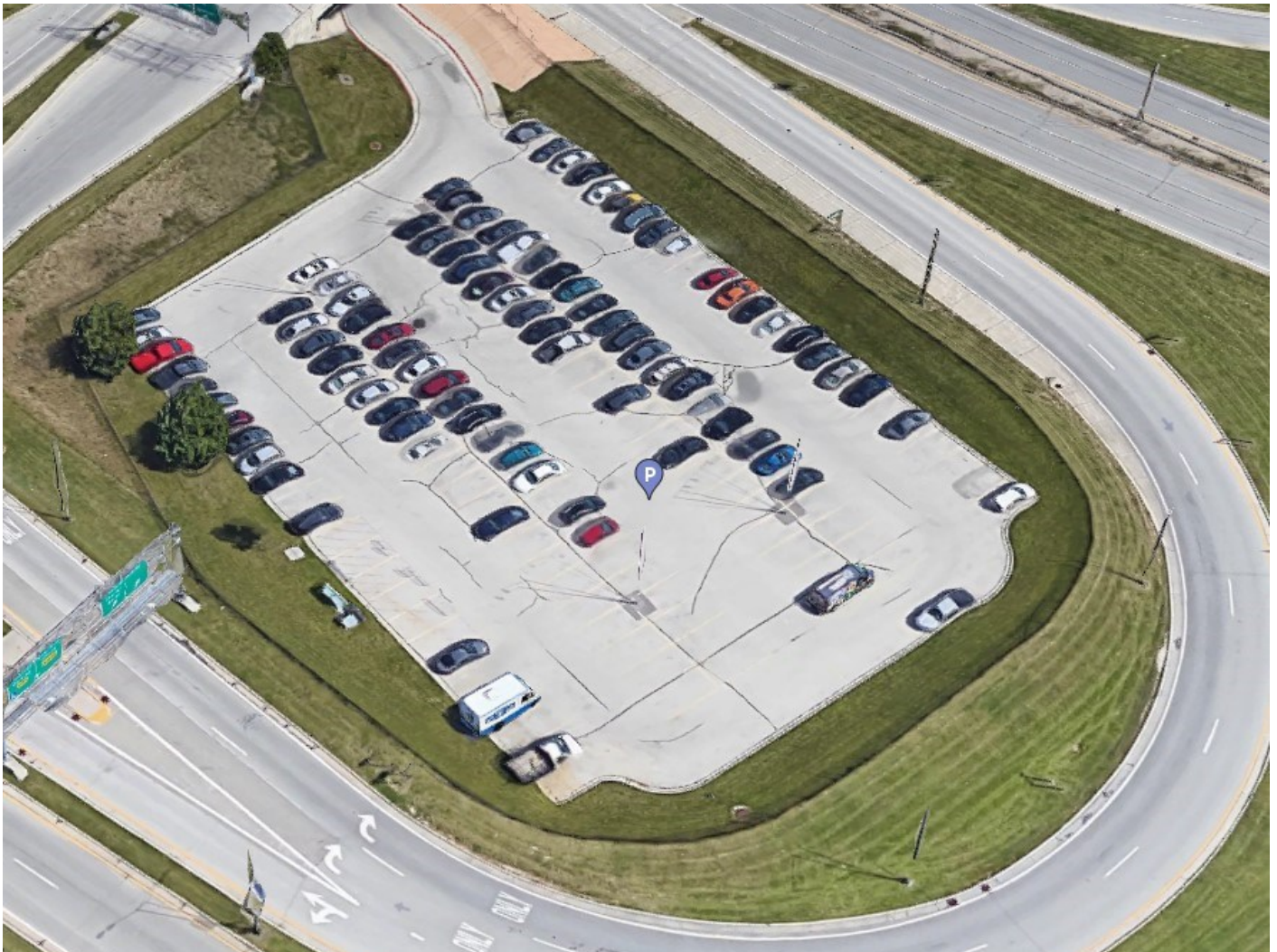
Photo 32: Logan Lot: Aerial photograph of Logan Lot, which depicts the asphalt lot cap, perimeter curb and gutter, and surrounding greenspace cap within the fence line around the property. Aerial imagery (2023).
